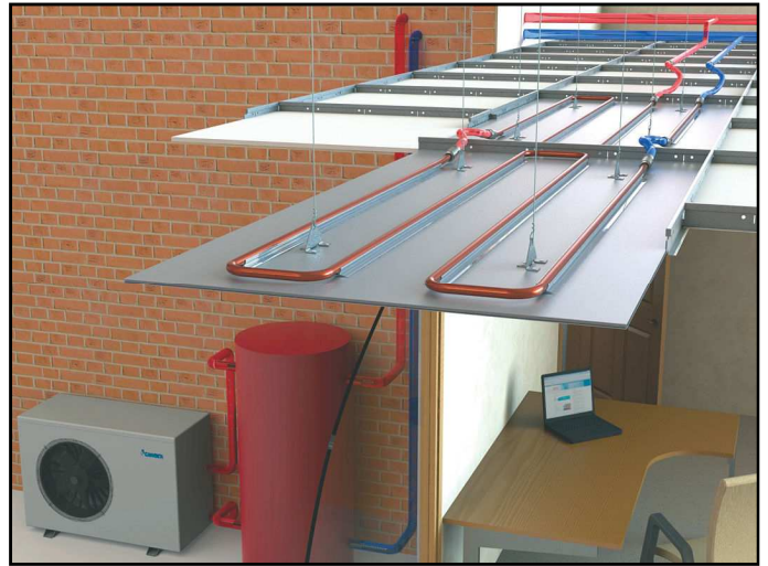
Radiant Panel / Heat Pump - Typical Installation
