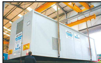
Loading Plant Room Within Works
