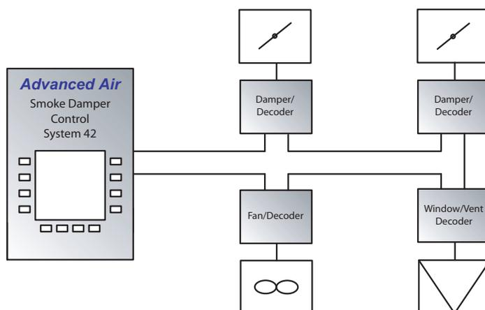
The control panel will be programmed to meet the exact requirements of the smoke management philosophy devised for the specific project. The instructions for each zone and damper are loaded into the panel via a lap-top computer during commissioning.
