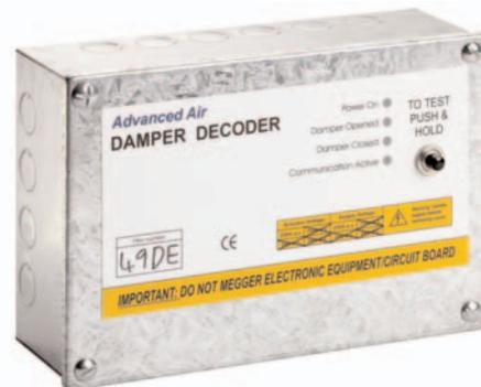
The decoder controls the main voltage to the damper actuator ( 230vac or 24v) instructing the damper to open or close according to the information received from the main panel. At the same time the position of the damper is monitored by the decoder. This information is constantly being sent back to the main panel to show the status of each damper on the system.
